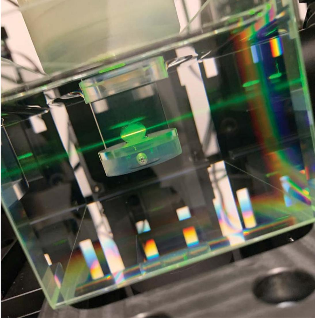
*A cleared mouse brain is secured to a sample holder (below) in preparation for imaging. Laser light is formed into a sheet and passed through the sample, which is now immersed in a liquid-filled chamber (left). A specialized lens is carefully calibrated into place for the three-dimensional imaging of the sample (bottom).*
