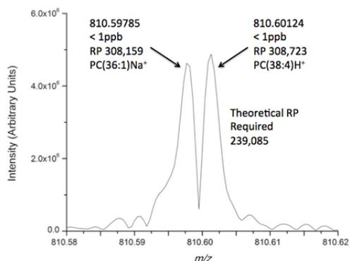
Figure 1. FT-ICR data acquired from rat brain highlighting the benefit of high-mass resolution and high-mass accuracy.
