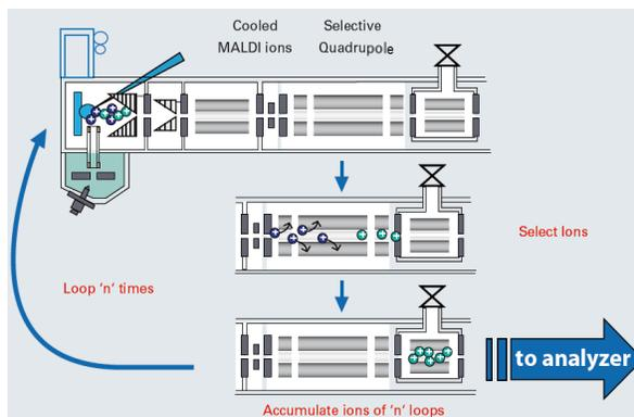
Figure 1. Schematic of CASI workflow where target ions are selected and enriched in the collision cell.
